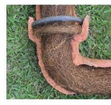
(Left) Tree roots can clog pipes, causing drainage problems and local flooding.
